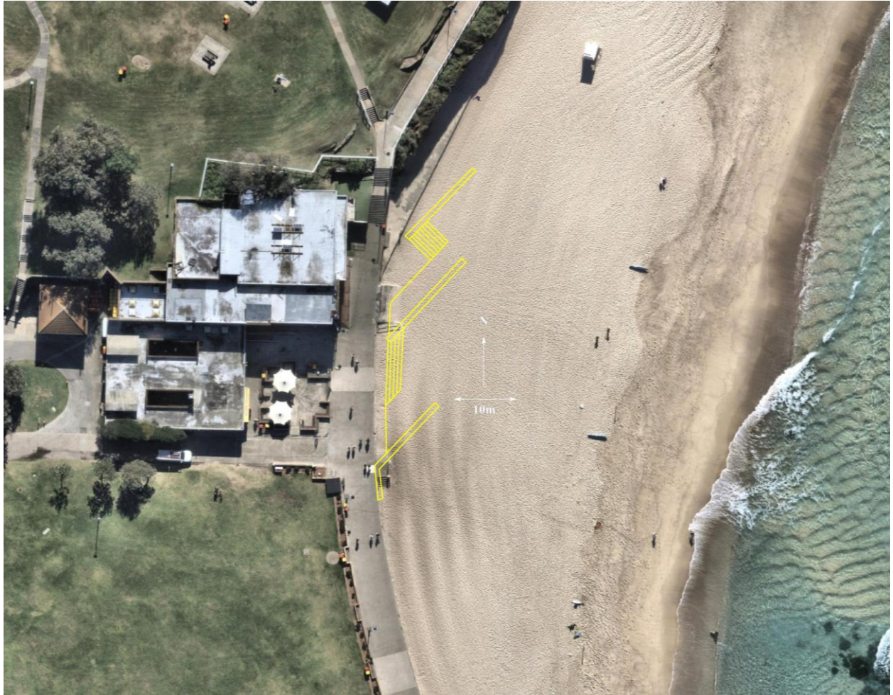
Figure 12: Alignment of proposed seawall, ramps and stairs at Bronte SLSC (aerial photograph taken 1 May 2023)
