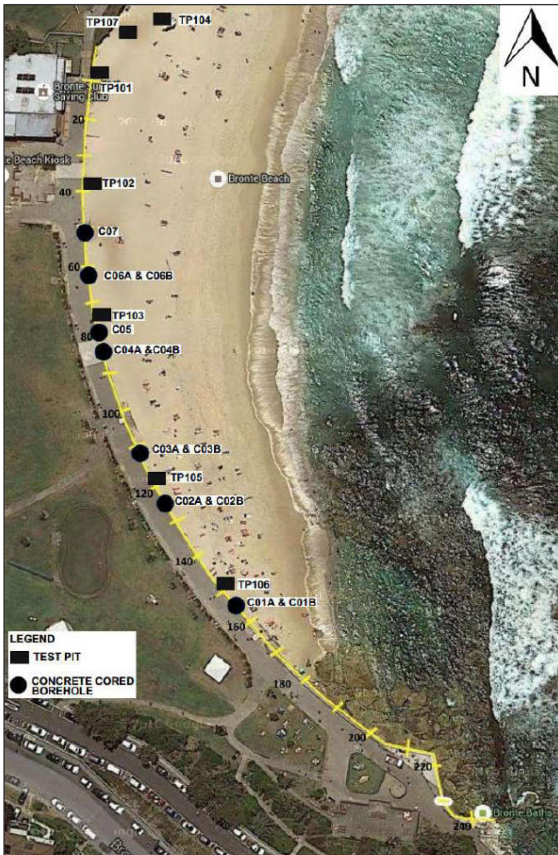
Figure 4-3 Seawall chainages and test pit and seawall coring locations (ARUP, 2016)
